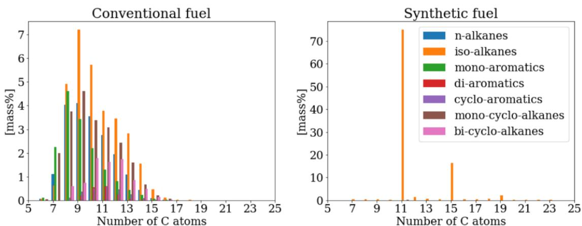
Figure 26. Comparison of the chemical composition of conventional and synthetic fuel.
