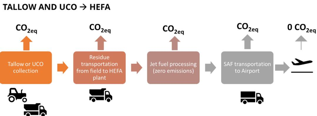
Figure 13. Lifecycle system boundary for tallow-based and UCO-based SAF using HEFA technology.
