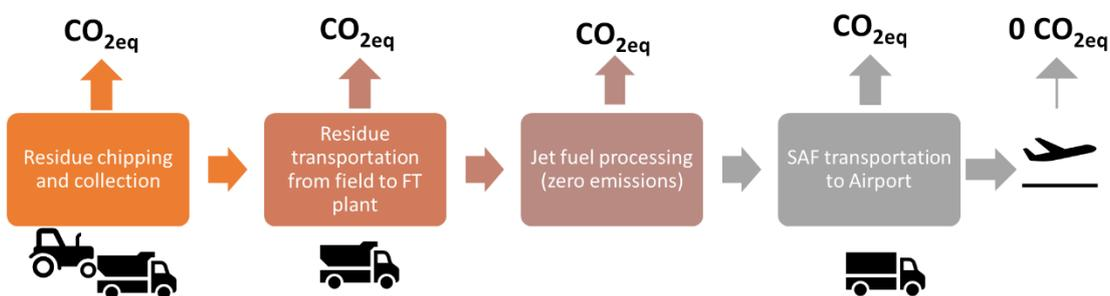
Figure 16. Lifecycle system boundary for forestry residue-based SAF using Fischer-Tropsch technology.
