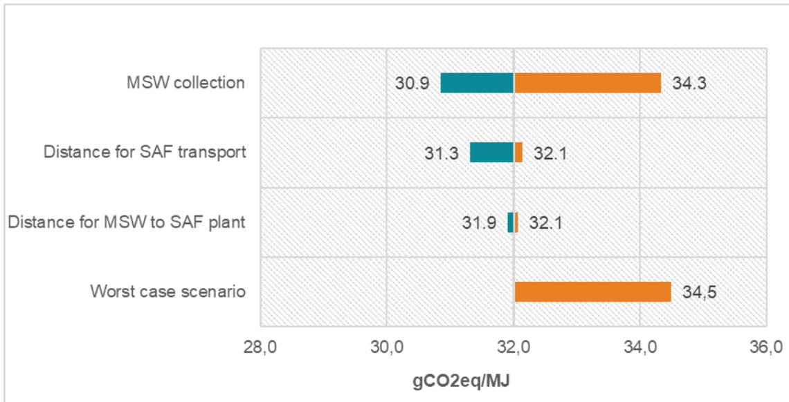
Figure 22. Sensitivity analysis of transport stages for FT-based SAF derived from municipal solid waste.
