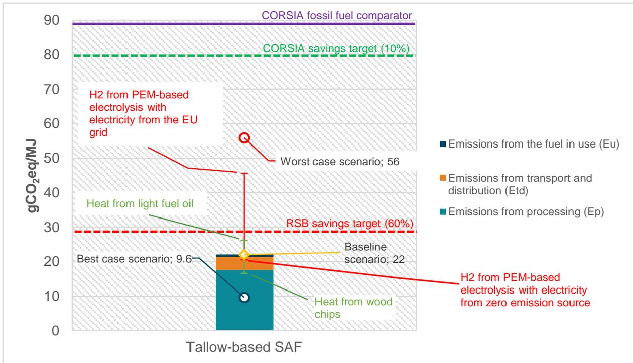
Figure 14. Breakdown lifecycle GHG emissions and sensitivity analysis for HEFA SAF production using tallow; point of origin is defined at the rendering plant.
