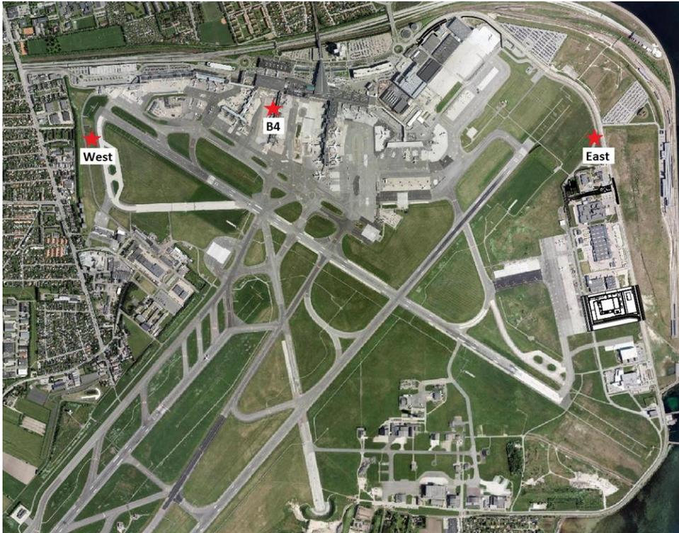
Figure 23. Copenhagen Airport and the locations of the airport's air quality monitoring stations (red stars): Station West (NO, NO<sub>2</sub>, PM<sub>2.5</sub>, BC and UFP), Station East (NO, NO<sub>2</sub>, PM<sub>2.5</sub>) and the apron station, Station B4 (NO, NO<sub>2</sub>, BC and UFP) (Ellermann, et al., 2012).
