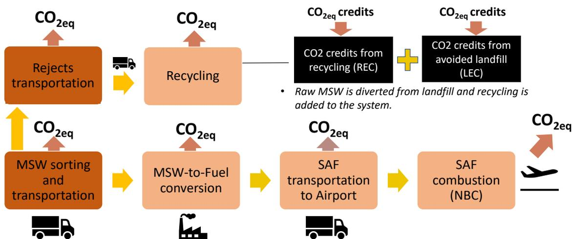
Figure 18. Lifecycle system boundary for municipal solid waste-based SAF using Fischer-Tropsch technology.
