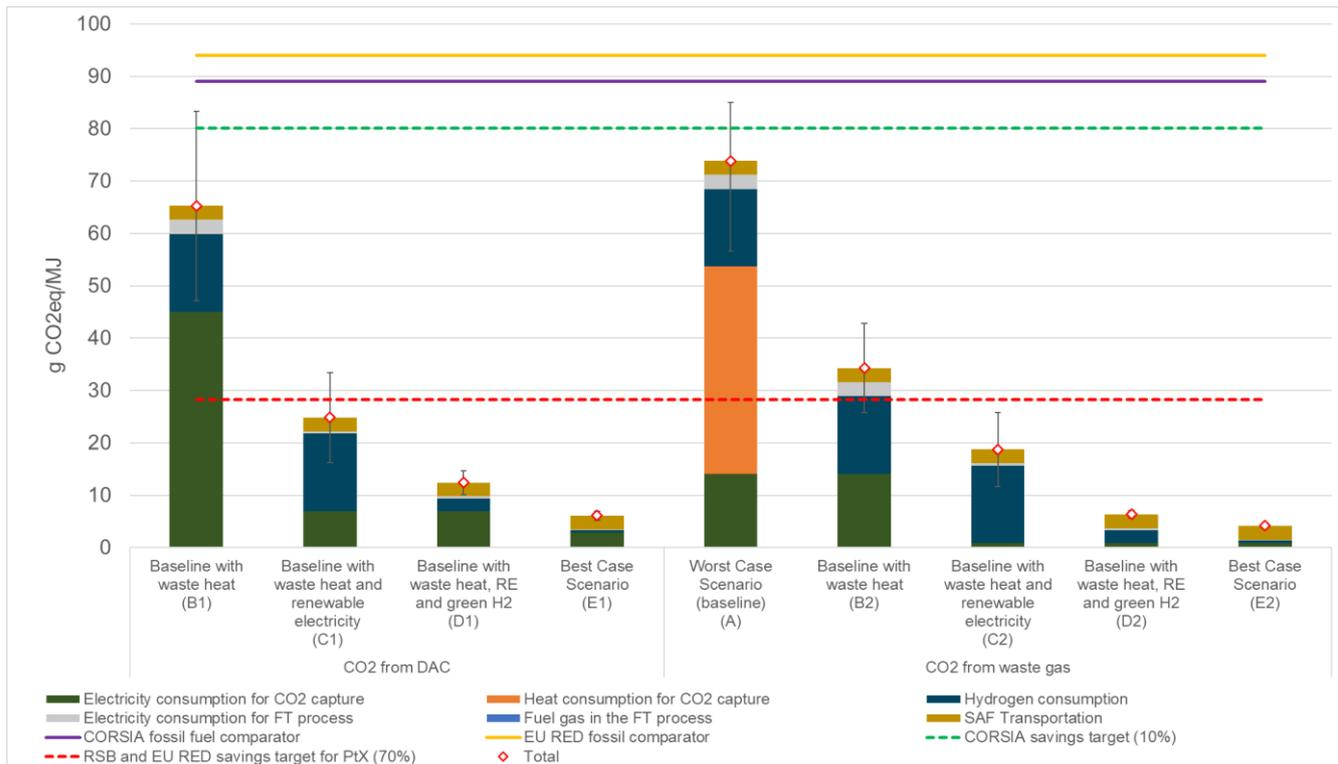
Figure 6. Breakdown lifecycle GHG emissions and sensitivity analysis for PtL SAF production.
