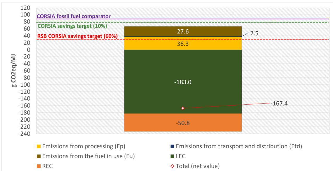
Figure 19. Breakdown lifecycle GHG emissions for FT-based SAF derived from municipal solid waste.
