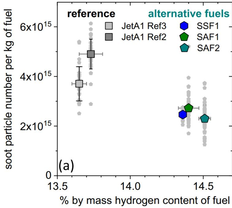
Figure 25. Soot particle emissions at cruise conditions for a conventional Jet A-1 fuel and low-aromatic SAF blends
