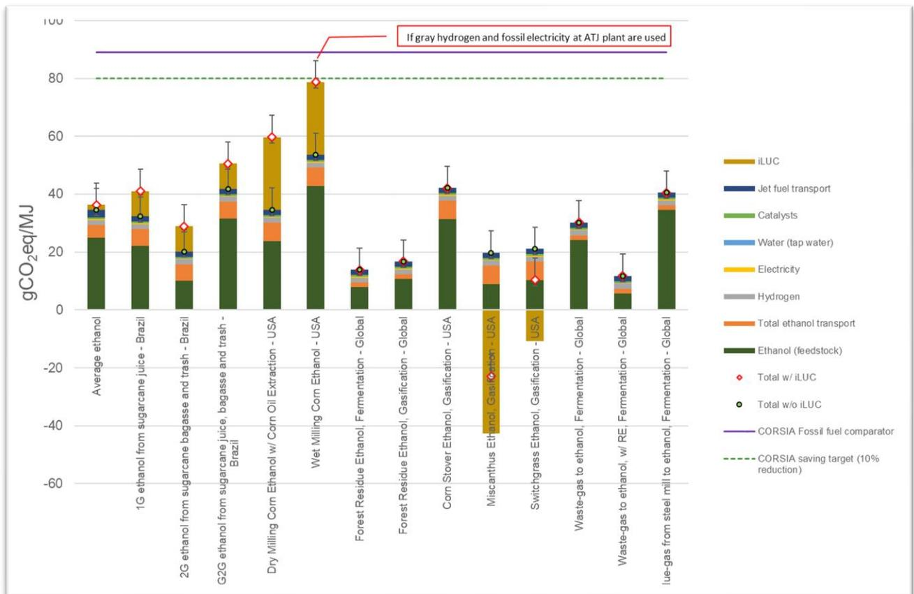
Figure 9. Breakdown lifecycle GHG emissions and sensitivity analysis for alcohol-to-jet SAF production using different ethanol types.
