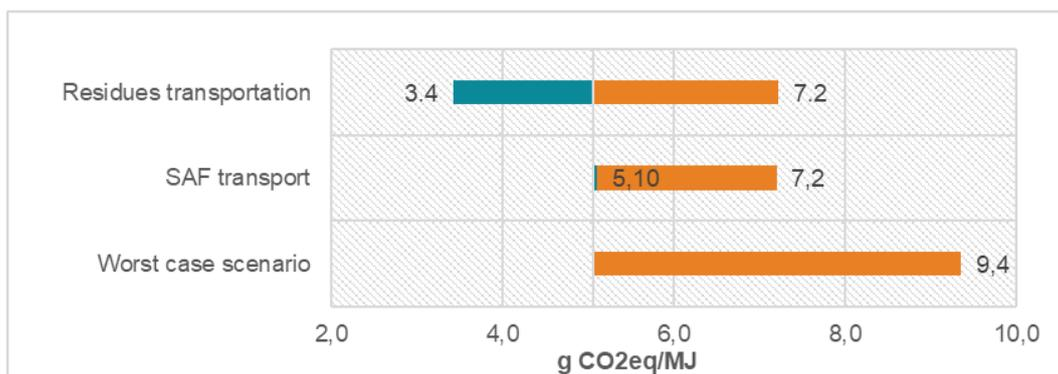
Figure 21. Sensitivity analysis of transport stages for FT-based SAF derived from forest residue.
