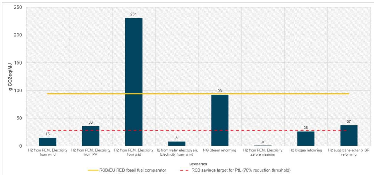
Figure 5. Sensitivity analysis for LCA GHG emissions of hydrogen produced from different pathways.
