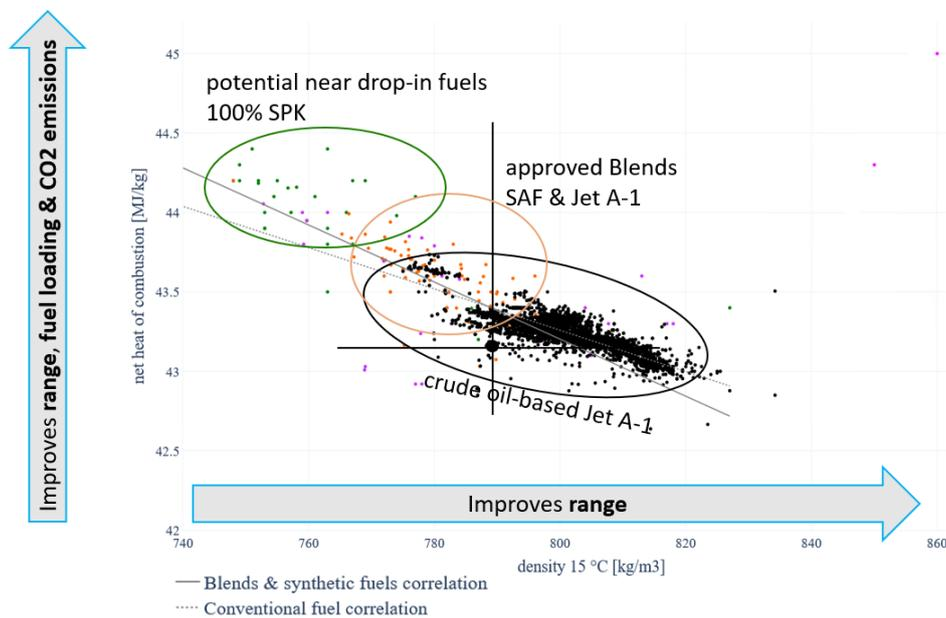
Figure 27. Net heat of combustion over density for a wide range of conventional jet fuels (black), SAF blends (orange) and neat SAFs (green)
